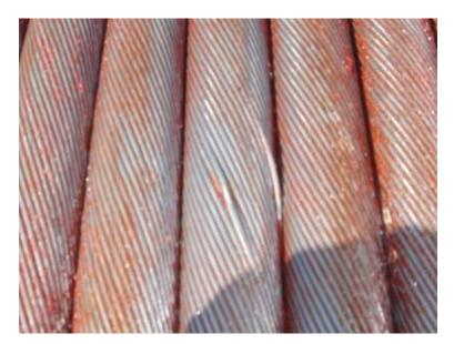
During BOS tests, the first failure of the sample was the breaking of a 24AWG conductor after 13429 cycles.
