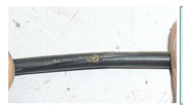
After inspection and analysis carried out by the supplier, it was stated that the design of the cable and the materials were not the cause of these defects.
